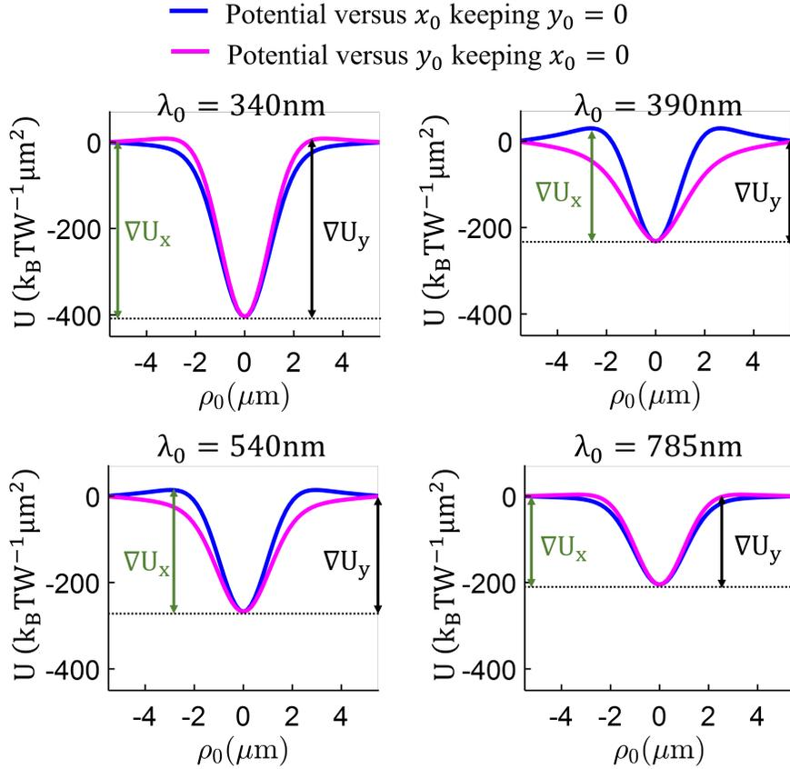
Fig. 7. Trapping potential computed as a function of the particle position  $(x_0, y_0)$  along  $(x_0$  with  $y_0 = 0$ ; blue line) and across  $(y_0$  with  $x_0 = 0$ ; magenta line) the nanorods of a nanostructured silver layer for several operation wavelengths. Local potential barriers along and across the nanorods are denoted as  $\Delta U_x$  and  $\Delta U_y$ , respectively. Other parameters are as in Fig. 2.
