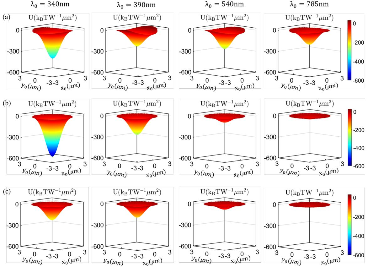
Fig. 6. Trap potential versus the position  $(x_0, y_0)$  of the particle when it is illuminated by a Gaussian beam oscillating at 340nm, 390nm, 540nm and 785nm operation wavelength. Results are computed when the particle is located above (a) a nanostructured silver layer; (b) a thin silver layer; and (c) bulk silver. Other parameters are as in Fig. 2.
