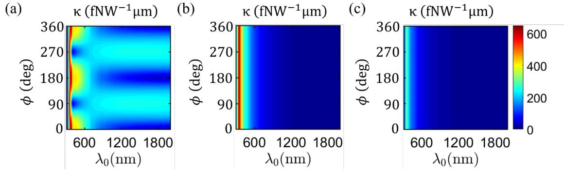
Fig. 8. Trap stiffness induced on a nanoparticle as a function of the wavelength ( $\lambda_0$ ) of the incident Gaussian beam and the polar angle ( $\phi$ ) defined with respect to the  $\hat{x}$ -axis in Fig. 1. Results are computed for a nanoparticle that is illuminated by a Gaussian beam and is located above (a) a nanostructured silver layer; (b) a thin silver layer; and (c) bulk silver. Other parameters are as in Fig. 2.
