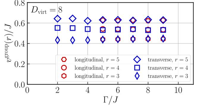
FIG. 22. Field dependence of the group velocity estimated from iPEPS simulations ( $D_{\text{virt}} = 8$ ) in 2D. For  $\Gamma/J < 5$ , we only show the group velocity estimated from the transverse correlations because the envelopes of longitudinal correlations become unclear for a weaker field.
