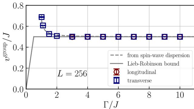
FIG. 11. Field dependence of the group velocity obtained by the LSWA in 1D. The exact Lieb-Robinson velocity  $v^{\text{LR}}/J = 1/2$  and the maximum group velocity  $v^{\text{SW}}/J = [1 + \sqrt{1 - (J/\Gamma)^2}]^{-1/2}/\sqrt{2}$  estimated from the spin-wave dispersion (see Appendix B 4) are shown as references. For  $\Gamma/J < 3$ , we only show the group velocity estimated from the transverse correlations because the envelopes of longitudinal correlations become unclear for a weaker field.
