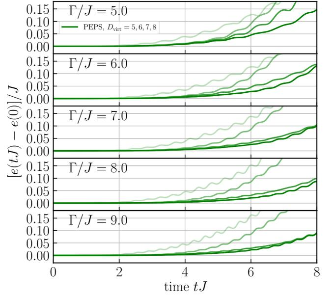
FIG. 2. Bond-dimension dependence of energy density obtained by iPEPS simulations. We consider the quench to  $\Gamma/J = 5, 6, 7, 8,$  and  $9$  and subtract the energy density at  $t = 0$ . The lines correspond to the time-dependent energy density for the bond dimensions  $D_{\text{virt}} = 5, 6, 7,$  and  $8$  (from lighter to darker). The energy is nearly conserved for  $D_{\text{virt}} \geq 6$  in a time frame  $tJ \in [0, 4]$ .
