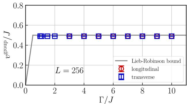
FIG. 6. Field dependence of the group velocity in 1D. The exact Lieb-Robinson velocity  $v^{\text{LR}}/J = 1/2$  is shown as a reference. For  $\Gamma/J < 3$ , we only show the group velocity estimated from the transverse correlations because the envelopes of longitudinal correlations become unclear for a weaker field.
