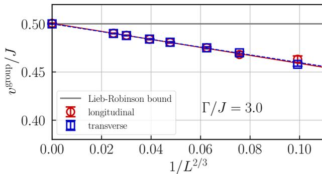
FIG. 7. Size scaling of the group velocity in 1D. The group velocity is well fitted by  $1/L^{2/3}$  with  $L$  being the length of a chain and is extrapolated to the value of the exact Lieb-Robinson velocity  $v^{\text{LR}}/J = 1/2$ .
