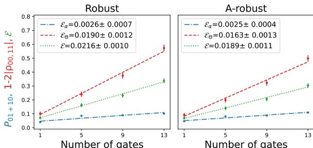
FIG. 5. Gate-error measurement of the robust and A-robust gate by applying repeated gate sequences. The blue (dash-dot), red (dashed) and green (dotted) lines and dots are the odd-parity population of  $|01\rangle$  and  $|10\rangle$  states, the parity contrast  $1 - 2|\rho_{00,11}|$ , and the measured gate error  $\mathcal{E}$ . Both gates have similar odd-parity populations, and the parity contrast of the A-robust gate outperforms that of the robust gate.
