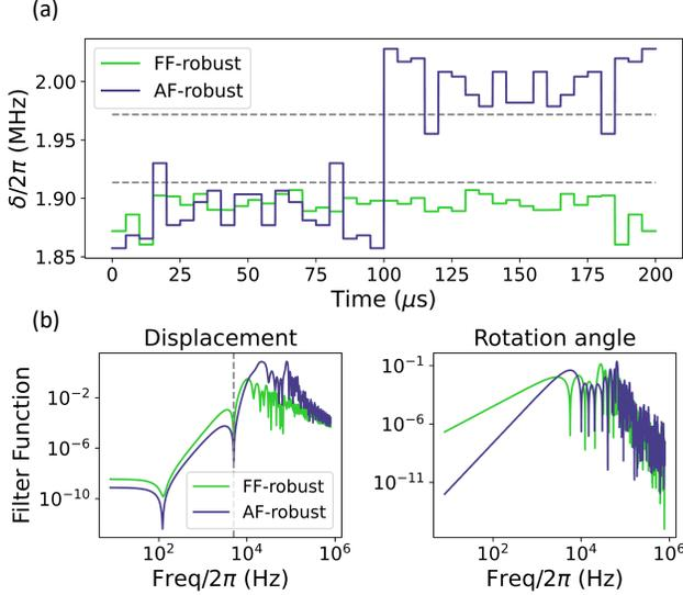
FIG. 7. (a) An example of 200- $\mu\text{s}$  pulses for two-ion discrete FF-robust and AF-robust FM  $XX(\pi/4)$  pulses. The carrier Rabi frequencies for the FF- and AF-robust pulses are 73.65 kHz and 100.36 kHz respectively. (b) The FFs of the pulses in (a). The pulses are optimized such that the displacement FF is suppressed near 5 kHz (dashed line).
