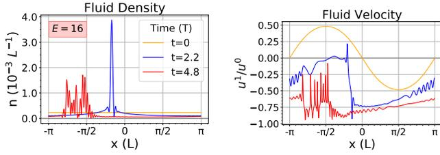
FIG. 2: Profiles of density  $n$  (left) and velocity  $u^1/u^0$  (right) at different times as functions of the position  $x$ , for an electric field  $E = 16$ , charge  $q = -1$ , mass  $m = 64$ , and initial maximum velocity  $u_{\max} = 0.55$ . The mesh size is  $N = 4096$ ,  $\epsilon = 2\pi/N$ ,  $T$  is an arbitrary time unit and  $L$  is an arbitrary length unit.
