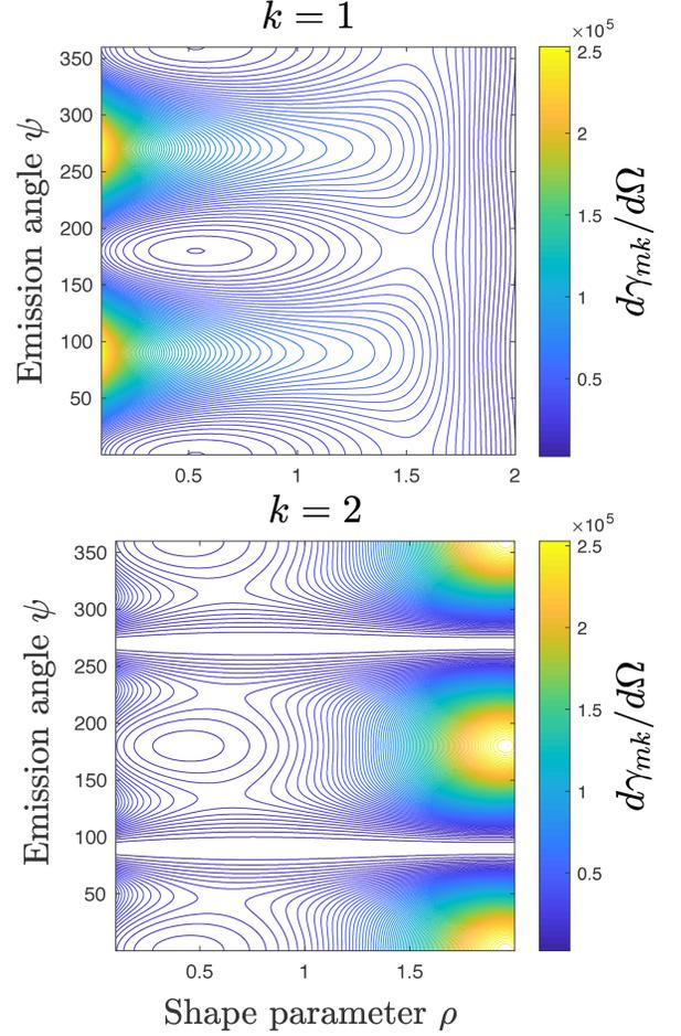
FIG. 5. Contour plots of curvature induced shift in the radiation pattern associated with the decay of plasmons excited on the cylindrical surfaces for the specified modes  $(m, k) = (0, 1)$  (up) and  $(m, k) = (0, 2)$  (down), and for different shape parameter  $\rho$  and varying emission angle  $\psi$  (see Eq. (51)).
