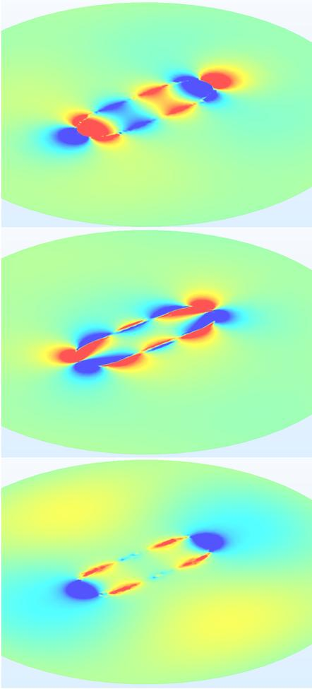
FIG. 7. Field component distribution  $E_x$  (top),  $E_y$  (middle),  $E_z$  (bottom) engendered in the nanoparticle by two dipoles symmetrically placed along the long axis of the nanoparticle. The dipoles emit at a wavelength of 535 nm with their moments parallel to the  $z$  axis.
