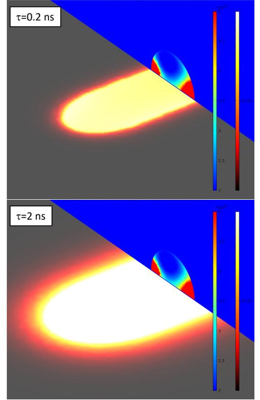
FIG. 11. Temperature distribution at  $t = 0.2$  ns (top) and  $t = 2$  ns (bottom) in the substrate plane due to energy losses in the nanoparticle. The energy loss density is visualized for an interacting field at a wavelength of 642 nm, corresponding to the plasmon excitation along the long axis of the nanoparticle.
