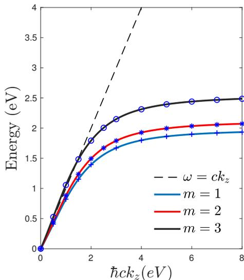
FIG. 2. Energy dispersion of the first three surface plasmon modes excited on a cylinder of radius  $\rho = 50$  nm. The cylindrical domain is modeled as a Drude material (see Appendix VIII A) bounded by vacuum.
