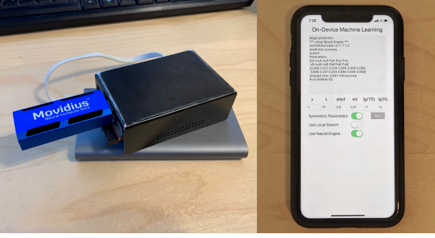
FIG. 1. Left: Raspberry Pi 3 single-board computer equipped with an Intel Movidius neural compute stick. Right: A smartphone (iPhone XR) running parameter prediction for a QKD protocol with an on-device neural network. In the same app one can also choose to run local search on the device (and compare its running time to that of neural networks).
