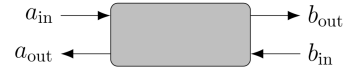
FIG. 2: Input and output fields coupled to a two-port black box quantum network. The input and output operators are continuous mode (as functions of frequency \omega ) annihilation operators, satisfying canonical commutation relations [32]. Here the mode a_{\text{in}}(\omega) carries the single-photon input state, the reflected mode is described by a_{\text{out}}(\omega) , and the output mode b_{\text{out}}(\omega) contains the excitation energy if the input energy successfully traversed the network (and may serve as input to the next part of the photo detection process, e.g., amplification, see Ref. [12]). b_{\text{in}}(\omega) may contain thermal excitations, but is never occupied by the photon we wish to detect.
