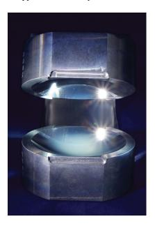
FIG. 8 (color). The ENS photon box (photograph by Michel Brune). The mirrors have a diameter of 5 cm and are 2.7 cm apart (for a clear view, they are more separated in this picture than in the actual experimental setup).
