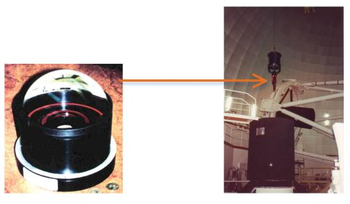
FIG. 32 (color). The F/1 wide-field CCD camera being mounted at the Anglo-Australian telescope.
