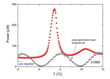
FIG. 5. Optical output power as a function of the operation temperature of the phase-preparation laser. The pulse-generation laser temperature is fixed, and the optical injection power is 50  $\mu$ W. Also shown are the optical power in the absence of optical injection (blue line) and the optical reflection of the injected light measured with the pulse-generation laser switched off (open circles), multiplied by a factor of 1000 for clarity.
