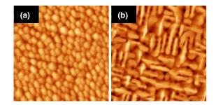
FIG. 3. Representative AFM scans for (a) Nb(100) and (b) Nb(110) surfaces. The scan size in both images is  $2 \ \mu m \times 2 \ \mu m$ .
