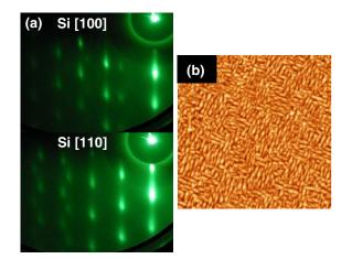
FIG. 5. (a) RHEED pattern for Nb(110)/Cu(100)/Si(100) along the Si[100] and Si[110] azimuths. (b) A representative 2  $\mu$ m × 2  $\mu$ m AFM scan for Nb films on the Cu template.
