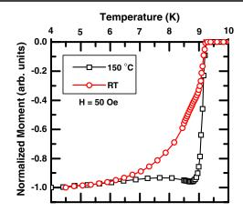
FIG. 6. Critical temperature transitions for films deposited at RT and 150°C.
