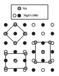
FIG. 1. Overlays of relaxed Nb lattices on an MgO(100) surface.
