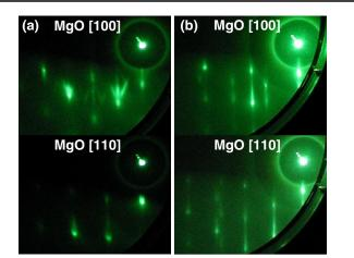
FIG. 2. RHEED patterns for (a) Nb(100)/MgO(100) and (b) Nb(110)/MgO(100) along the MgO[100] and MgO[110] azimuths.
