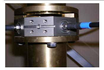
FIG. 15. (Color) Photo of the template positioned with pawns above the BPM block. The rod is positioned at the center of the BPM in X and Y by electric contacts with the template. Afterwards, the template is removed and the upper flange is delicately screwed on the BPM. Two half crown pieces are inserted under the rf joint to maintain an equal height.
