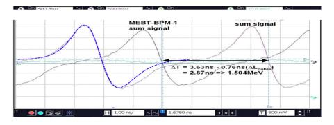
FIG. 5. (Color) Averaged sum of the four electrode signals obtained in the high energy section of SARAF. The dashed trace shows the response of a MATHEMATICA simulation using the same parameters as experimental conditions: a proton beam current of 4 mA at  $\beta = 0.06$ , the bunch base length is  $\pm 22^{\circ}$ , the acceleration frequency is 176 MHz, and the inner pipe radius is 15 mm.
