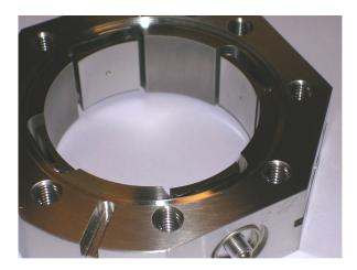
FIG. 9. (Color) An IPHI BPM (core, feedthrough, and assemblies) has been built by the French company PMB. The space between electrode and core is 2 mm with a tolerance of  $\pm 0.05$  mm. The four standard Metaceram 50  $\Omega$  feedthroughs are terminated by SMA connectors. During the brazing process the four electrodes have been positioned by using a template to align the axial symmetry.
