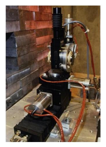
FIG. 10. (Color) Birefringent (quarter wave plate) Si crystal and goniometer.
