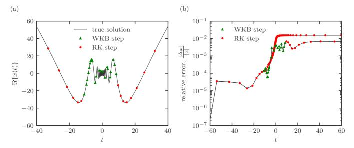
FIG. 2. Numerical solution of the burst equation with n = 40. A relative tolerance of  $10^{-3}$  was set, and the equation was solved from t = -2n to t = 2n.
