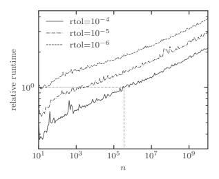
FIG. 5. Relative runtime of solving the burst equation from t = -2n to t = 2n, with n varying from  $10^1$  to  $10^{10}$ , and the relative tolerance "rtol" from  $10^{-4}$  to  $10^{-6}$ . The runtimes are referenced to the median of the n range and relative tolerance of  $10^{-4}$ , as indicated by the dotted lines.
