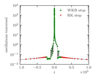
FIG. 3. Number of oscillations stepped over in a single step, while solving the burst equation with  $n = 10^5$ , and a relative tolerance of  $10^{-4}$ .
