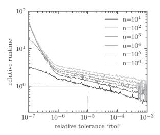
FIG. 6. Relative runtime of solving the burst equation, as a function of the relative tolerance set (with the absolute tolerance set to 0). The different curves show different values of n, proportional to the total number of oscillations traversed.
