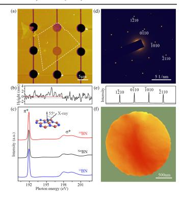
FIG. 1. (a) AFM image of a mechanically exfoliated  $1L^{10}BN$  suspended over Au/Si substrate with microwells and trenches. (b) AFM height of the 1L sample. (c) NEXAFS spectra in the B K-edge region of isotopically pure and natural BN at the incidence of 55°. (d) Selected area electron diffraction of a suspended  $1L^{10}BN$ . (e) The corresponding diffraction spot intensities and (f) the DF-TEM image.
