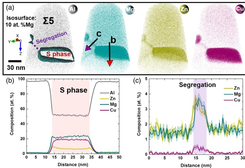
FIG. 3. APT analysis of the same  $\Sigma 5$  GB with the STEM analysis: (a) Atom maps of all elements; (b) Corresponding composition profile across the precipitate calculated along the red arrow; (c) Corresponding composition profile across the region between two precipitates calculated along the purple arrow.
