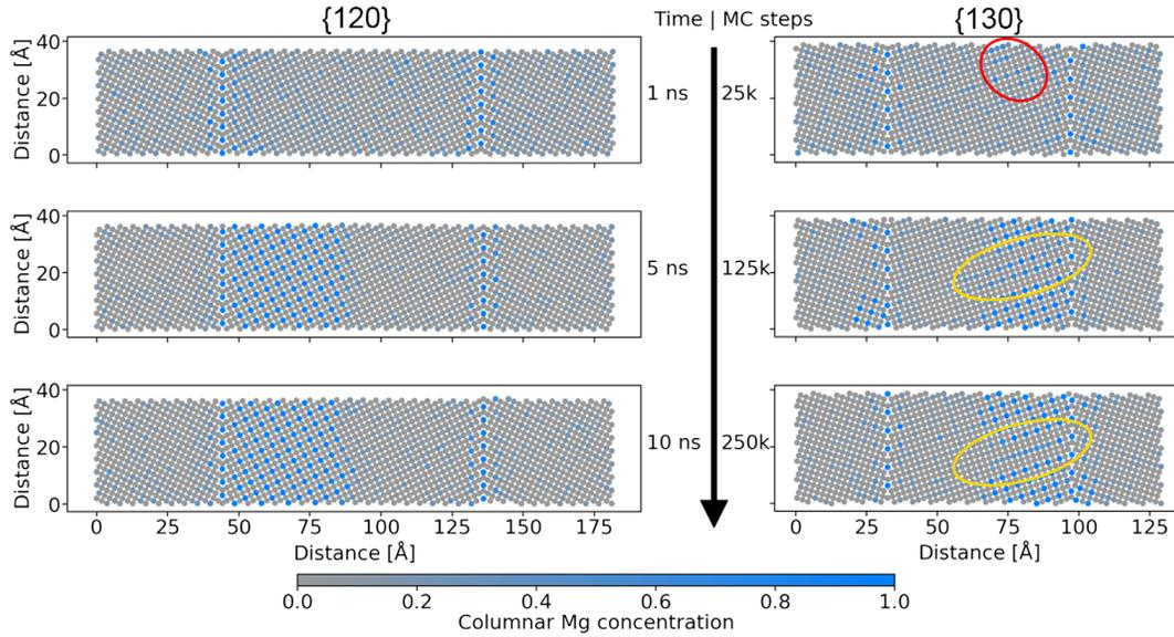
FIG. 4. VC SGC and MC-MD results for precipitate formation at  $\{120\}$  and  $\{130\}$  boundaries at  $25^\circ\text{C}$ . Results are shown in an  $\langle 001 \rangle$  projection and colored according to Mg concentration. Snapshots are shown from three points in time for each boundary. Red and yellow ovals are discussed in the text.
