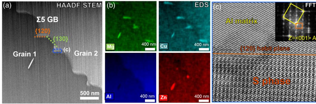
FIG. 2. (a) HAADF STEM image of a  $\Sigma 5$  GB in the as-quenched alloy; (b) EDS maps of the faceted GB showing Mg-Cu enriched precipitates; (c) HAADF STEM image of the precipitate highlighted by blue rectangle in (a), with inset the corresponding Fast Fourier transform (FFT) pattern.
