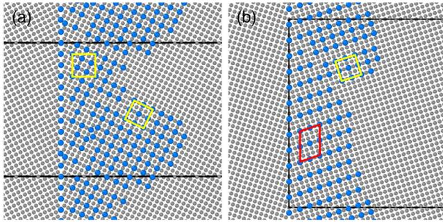
FIG. 5. Snapshots of Mg (large blue) segregation to the ideal  $\Sigma 5$  symmetric: (a)  $\{120\}$  and (b)  $\{130\}$  boundaries in Al (small gray). Yellow squares indicate domains with an  $\text{Al}_3\text{Mg}$  stoichiometry and similarly the red trapezoid indicates  $\text{Al}_5\text{Mg}$ . The black lines show periodic boundaries of the simulation domain (not all of which is shown).
