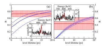
FIG. 1. Graphical determination of the lifetimes of the  $2^+$  (a) and  $4^+$  (b) excited states of <sup>84</sup>Ge (see text). The shaded area and the two thinner curves materialize the  $1\sigma$  uncertainty regions. The insets show the relevant regions of the gamma spectrum, with the shifted and unshifted photo-peak components marked with "S" and "U," respectively.
