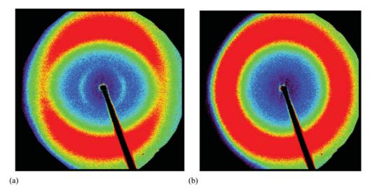
FIG. 3. (Color) X-ray scattering images from a magnetically aligned sample of CB7CB in the supercooled X phase at 86  $^{\circ}$ C. The incident x-ray beam is perpendicular to the page. Part (a) is with the field in the plane of the page, and (b) is with the sample rotated so that the original field direction is perpendicular to the page.
