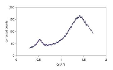
FIG. 4. (Color online) The azimuthally averaged scattering intensity determined for CB7CB in the aligned X phase at 86 °C as a function of the scattering vector, Q.
