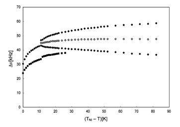
FIG. 13. The dependence of the quadrupolar splittings,  $\Delta \nu$ , on the shifted temperature  $(T_{\rm NI} - T)$  for the 1", 7" deuterons ( $\blacklozenge$ ) and for the low-intensity doublet ( $\blacksquare$ ) in the *N* and *N<sub>X</sub>* phases. The average of the two splittings for the 1" and 7" deuterons in the *N<sub>X</sub>* phase is shown as ( $\diamondsuit$ ).
