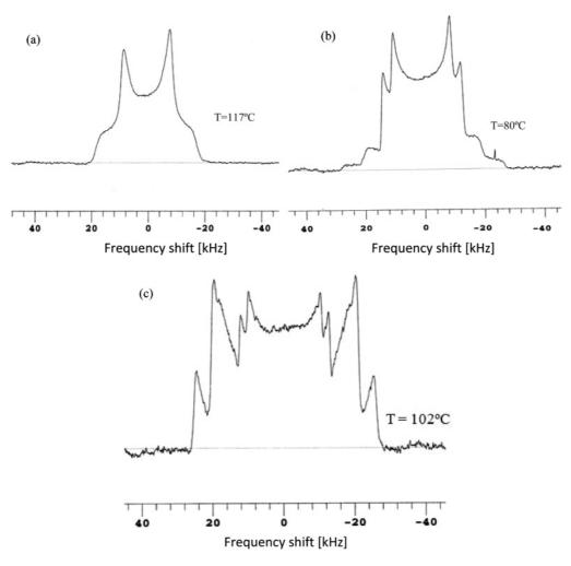
FIG. 11. The deuterium NMR spectra of CB7CB- $d_4$  (a) in the *N* phase at 117 °C randomly distributed in the CPG, (b) in the supercooled  $N_X$  phase at 80 °C randomly distributed in the CPG, and (c) in the partially random distribution for the bulk sample of the  $N_X$  phase at 102 °C. The vertical axis is the spectral intensity in arbitrary units, while the horizontal axis is a scale of frequency shifts relative to the center of the spectra.
