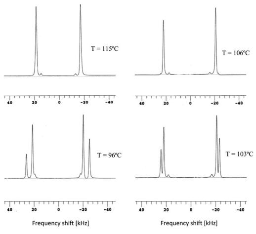
FIG. 12. The deuterium NMR spectra of CB7CB- $d_4$  aligned by a magnetic field of 7.05 T. From top, clockwise: nematic phase (115 °C), nematic phase (106 °C),  $N_X$  phase (103 °C), and  $N_X$  phase (96 °C). The vertical axis is the spectral intensity in arbitrary units, while the horizontal axis is a scale of frequency shifts relative to the center of the spectra.
