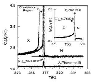
FIG. 5. Heat-capacity measurements for CB7CB in the region of the  $N_X$ -to-N phase transition. Cooling and heating runs are represented by full and empty symbols, respectively. The  $\delta$ -phase shift (arb. units) accounts for the narrow coexistence region.
