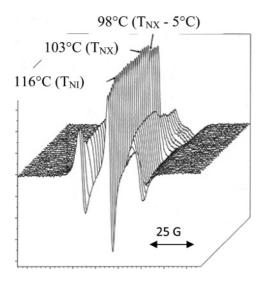
FIG. 10. A stack plot of the ESR spectra of a cholestane spin probe dissolved in CB7CB shown as a function of temperature. The vertical axis is a derivative of the spectral intensity in arbitrary units, while the horizontal axis is the scanned magnetic-field strength.
