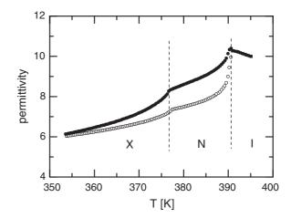
FIG. 6. The principal components of the permittivities, extrapolated to zero frequency, for CB7CB shown as a function of temperature: parallel ( $\varepsilon_{para} = \bullet$ ) and perpendicular ( $\varepsilon_{perp} = o$ ) components.
