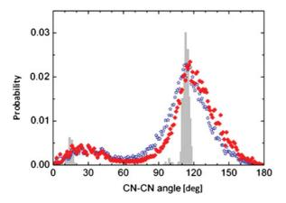
FIG. 14. (Color online) The probability distributions for the angle between the terminal mesogenic groups of CB7CB, calculated for the uniaxial nematic phase at two different values of the order parameter  $S_{zz}$ . Results for the continuous torsional potential are given for  $S_{zz} = 0.30$  (open stars) and  $S_{zz} = 0.46$  (filled diamonds). For comparison, the distribution obtained for the RIS model is shown as a histogram.
