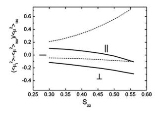
FIG. 15. Results for the parallel and perpendicular mean-square dipole moments of CB7CB calculated as a function of the order parameter,  $S_{zz}$ . Solid lines show the results obtained by MC sampling of conformations generated with CTP, while the dashed lines are those obtained by MC sampling of RIS conformers.
