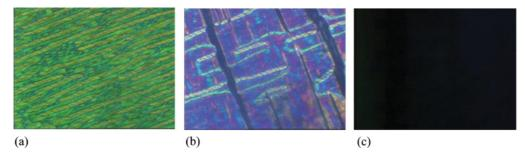
FIG. 9. (Color online) The effect of a voltage applied (10 Hz triangular) across a planar aligned sample (100°C) of the  $N_X$  phase of CB7CB on its optical texture. (a) Zero field, (b) field of 4 MV m<sup>-1</sup>, and (c) after the electric field is removed from the fully switched state.
