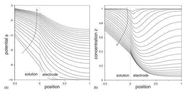
FIG. 4. Capacitive response of porous electrode to step change in electrode potential as function of time and position. Arrow shows the direction of time, 0.001 < t < 0.5. Parameter settings in the text. (a) Electrostatic potential,  $\phi$ . (b) Salt concentration, c.
