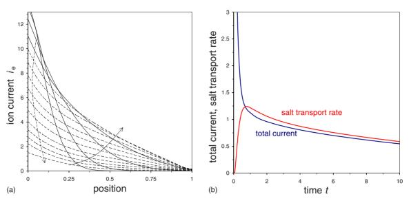
FIG. 5. (Color online) (a) Ion current profiles in the electrode as function of time. Arrows show the direction of time (0.001 < t < 0.5; first solid curves, next dashed curves). Ion current at position x=0 equals the total current. (b) Total current versus time t, and salt transport rate evaluated at the outer edge of the SDL.
