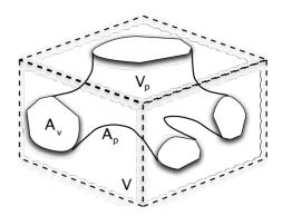
FIG. 6. Sketch of a macroscopic volume element of volume V containing a pore space of volume  $V_p$  and internal surface area  $A_p$ , which intersects the volume element with cross-sectional area  $A_p$ .
