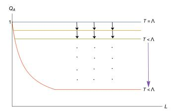
FIG. 8. A schematic depiction of the entanglement entropy in the Schwarzschild-AdS spacetime, normalized by the maximal value of entropy in the subregion,  $Q_A = S_A/S_{A,\max}$ , and depicted as a function of the size L of subregion A; see Eq. (20). The scales of the axes are arbitrary. As the mass of the black hole is lowered (the temperature T of the holographic theory is reduced from the cutoff  $\Lambda$ ),  $Q_A$  deviates from 1 in a specific manner.
