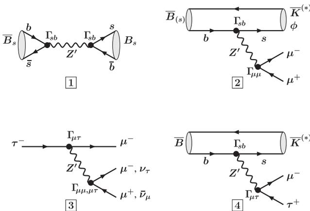
FIG. 1. Feynman diagrams illustrating the steps (1)–(4) of our analysis (see text). The diagrams display the dominant  $Z'$  contribution to  $\bar{B}_s - B_s$  mixing,  $\bar{B} \rightarrow \bar{K}^{(*)} \mu^+ \mu^-$ ,  $\bar{B}_s \rightarrow \phi \mu^+ \mu^-$ ,  $\tau \rightarrow 3\mu$ ,  $\tau \rightarrow \mu \nu \bar{\nu}$  and  $\bar{B} \rightarrow \bar{K}^{(*)} \tau^+ \mu^-$ .
