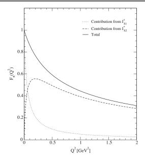
FIG. 2. Scalar pion form factor (solid line) and its valence (dotted line) and nonvalence (dashed line) contributions for  $0 \le Q^2 \le 2$  GeV<sup>2</sup> region.
