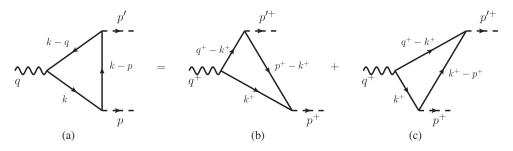
FIG. 3. One-loop Feynman diagrams that contribute to  $\gamma^*(q) \rightarrow \overline{\mathcal{M}}(p) + \mathcal{M}(p')$ . The covariant diagram (a) is the same as the sum of the two LF time-ordered diagrams (b) and (c).
