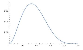
FIG. 1. A plot of the potential for the critical first order point, Eq. (96). The masses squared is nonzero about the perturbative vacuum, q = 0, but vanishes about the confining vacuum, q = 1/2.
