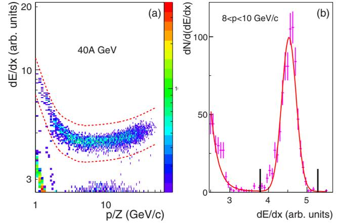
FIG. 2. (a) Energy loss  $dE/dx$  measured in the MTPC as a function of rigidity for charged tracks from central Pb + Pb collisions at 40A GeV. The dashed curves indicate the PID cut boundaries used for selection of  $^3\text{He}$ . (b) Distribution of  $dE/dx$  in the momentum interval  $8 < p < 10$  GeV/c. A fit of a Gaussian signal plus background is shown by the solid curve. Black vertical lines indicate the selection window for  $^3\text{He}$ .
