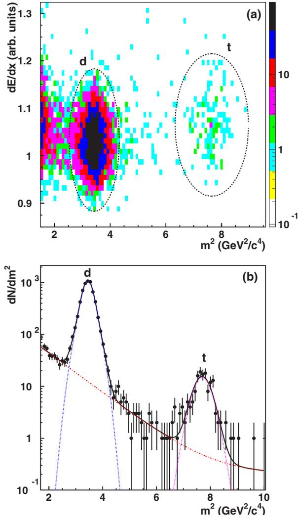
FIG. 1. (a) Energy loss  $dE/dx$  versus mass squared from Pb + Pb at 20A GeV for the momentum interval  $6 < p < 8$  GeV/c. Deuteron and triton candidates are selected within the  $3\sigma$  particle identification (PID) ellipses indicated by the dashed lines. (b) Mass-squared distribution after a  $dE/dx$  upper limit cut (see text). The solid line indicates the best fit with two Gaussians (the dotted lines) and the background (the dash-dotted line).
