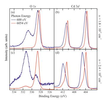
FIG. 1. (Color online) Comparison of HAXPES and SXPES taken using photon energies of 6054 and 600 eV, respectively. (a) O 1s, (b) Cd 3d for the annealed sample ( $n=1.8\times10^{19}~{\rm cm}^{-3}$ ) and (c) O 1s, (d) Cd 3d for the as-grown sample ( $n=2.4\times10^{20}~{\rm cm}^{-3}$ ).
