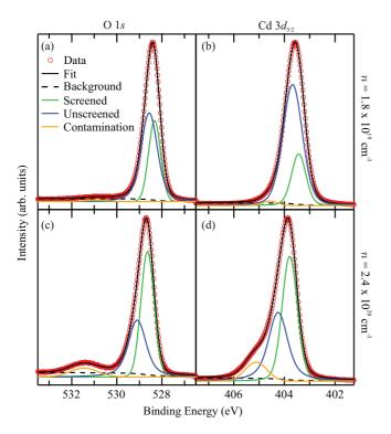
FIG. 4. (Color online) HAXPES spectra and fits for (a) O 1s, (b) Cd  $3d_{5/2}$  for the annealed sample ( $n=1.8\times10^{19}~\rm cm^{-3}$ ). (c) O 1s, (d) Cd  $3d_{5/2}$  for the as-grown sample ( $n=2.4\times10^{20}~\rm cm^{-3}$ ). Fits were preformed using three Voigt line shapes and a Shirley background, the assignment of the peaks is discussed in the text.
