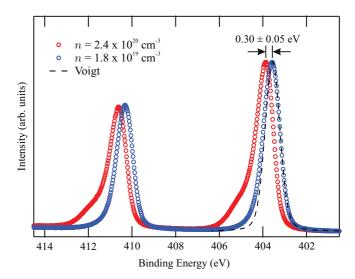
FIG. 3. (Color online) Cd 3d spectra shown for the as-grown  $(n = 2.4 \times 10^{20} \, \mathrm{cm}^{-3}, \, \mathrm{red})$  and annealed  $(n = 1.8 \times 10^{19} \, \mathrm{cm}^{-3}, \, \mathrm{blue})$  samples. A symmetric Voigt peak shape is also shown as a reference to allow the asymmetry to be observed.
