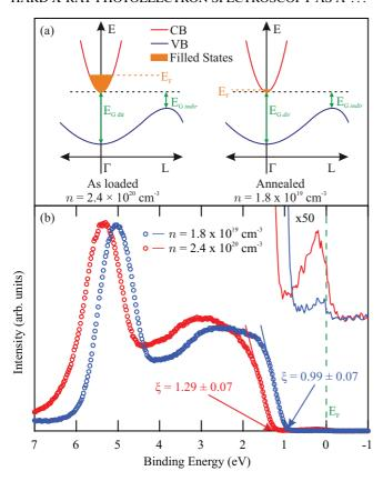
FIG. 2. (Color online) (a) A band schematic for a high and low carrier concentration, illustrating the band filling and indirect band gap. (b) HAXPES valence band spectra for the as-grown ( $n = 2.4 \times 10^{20}$  cm<sup>-3</sup>, red) and annealed ( $n = 1.8 \times 10^{19}$  cm<sup>-3</sup>, blue) samples. Extrapolations of the VB leading edge are shown. Magnified (×50) and offset spectra (solid line) are also shown allowing the CB intensity just below the Fermi level ( $E_F$ ) to be visible.
