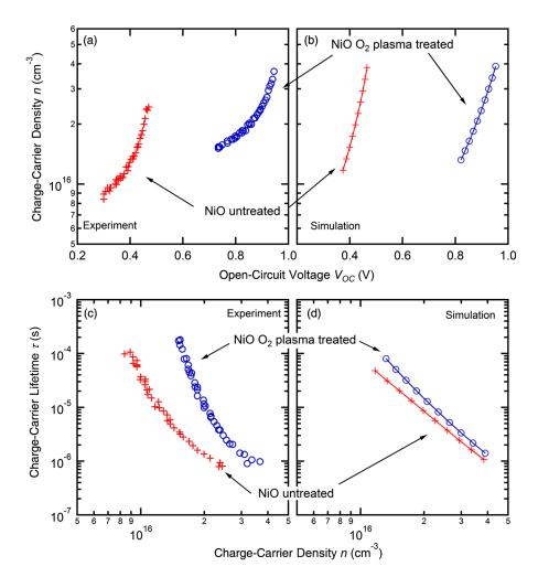
FIG. 4. Measured (a),(c) and simulated (b),(d) charge-carrier density n as a function of  $V_{\rm OC}$  as measured from CE (a),(b) and charge-carrier lifetime  $\tau$  as measured from TPV (c),(d).  $O_2$  plasma-treated NiO (open circles) and untreated NiO (crosses).
