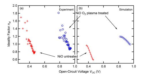
FIG. 3. Measured (a) and simulated (b) ideality factors at different open-circuit voltages for an untreated NiO-based device (crosses) and a plasmatreated NiO-based device (open circles).
