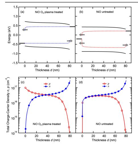
FIG. 2. Simulated band diagrams and total carrier densities as a function of active-layer thickness for O2 plasma-treated NiO (a),(c) and untreated NiO (b),(d). Band diagrams (a),(b) show the mobility edge (solid lines) and quasi-Fermi-level splitting (dashed lines), while arrows demonstrate the presence of surface recombination. (c) and (d) show electron carrier densities (filled circles) and hole carrier densities (empty circles). The anode contact is located at 0 nm and the cathode at 80 nm.
