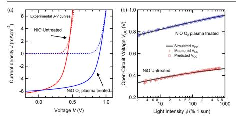
FIG. 1. (a) Dark (dashed lines) and illuminated under AM1.5 (solid lines) J-V curves for devices made on untreated and  $O_2$  plasma-treated NiO. (b) Opencircuit voltage versus illumination for both devices (crosses) as well as predictions based on experimental measurements of the density dependence of charge-carrier lifetime  $\tau_n$  (open symbols) and simulations based on 1D drift-diffusion modeling (solid lines).
