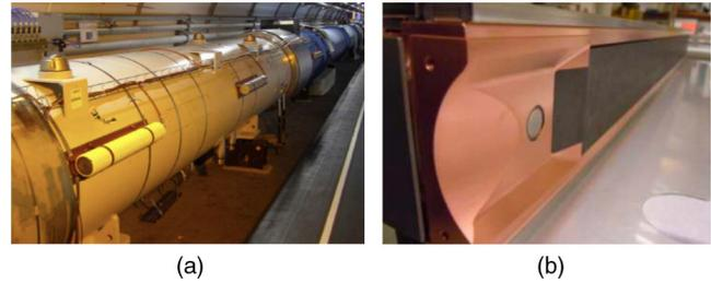
FIG. 3. (a) BLM detectors installed in the LHC and (b) BPM detectors installed in collimator jaws.
