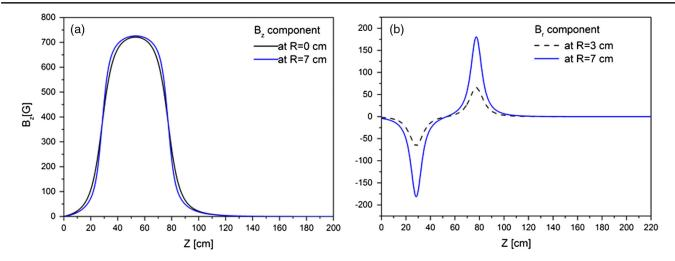
FIG. 3. Simulated magnetic fields used in the simulation for a 201 A driving current on the extraction solenoid when the bucking coil current is chosen to minimize the on axis magnetic field at the velvet cathode; (a)  $B_z$  at R = 0 cm (black line) and R = 7 cm (blue line) as a function of Z; (b)  $B_r$  component at two different radii: at R = 3 cm (black dashed line) and R = 7 cm (blue line).
