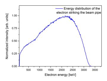
FIG. 8. Simulated time integrated energy distribution of the loss electrons striking the pipe.
