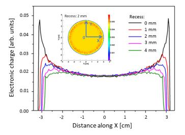
FIG. 5. Simulated electron beam profile at the cathode, along X at Y = 0, on the flattop voltage for a 3.175 cm cathode radius for five recess values ranging from 0 to 4 mm. The inserted image is a 2D plot of the simulated beam distribution at the cathode for a 2 mm recess.
