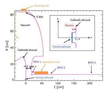
FIG. 1. Geometry used for simulating the beam dynamics inside an injector of an induction accelerator. BPM (for beam positioning monitor) indicates the location of the current sensors. The inset is a zoom in the diode region.
