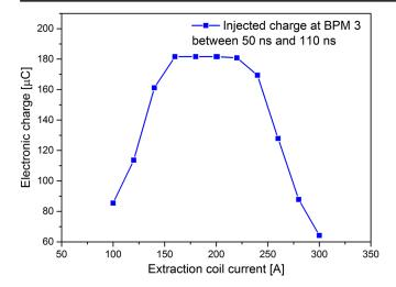
FIG. 9. Simulated electronic charge at BPM 3 integrated over 50 and 110 ns corresponding to the quasiflat part of the voltage pulse.
