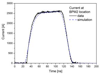
FIG. 6. Experimental and simulated currents at the BPM 2 location for the new 3.175 cm radius velvet cathode and a 201 A driving current.
