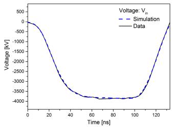
FIG. 2. Typical measured voltage on EPURE axis-1 (black) and simulated voltage (dashed blue) used as an inlet boundary in the simulation ( $V_{in}$  in Fig. 1).
