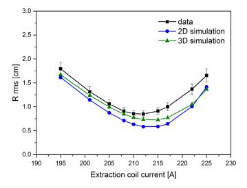
FIG. 10. Comparison of rms beam radii at BPM 3 for various extraction coil currents: measured (black squares) and simulated using an axisymmetric 2D geometry (blue circles) and a Cartesian 3D geometry (green triangles).
