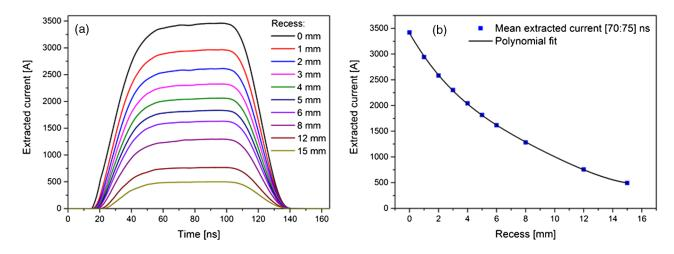
FIG. 4. (a) Simulated electron beam current at BPM 1 as a function of time for different recess values. (b) Simulated mean beam current over [70–75] ns range as a function of recess (blue square) and fourth order polynomial fit (black curve): current = 3408.08 - 491.40(recess) + 47.76(recess)<sup>2</sup> - 3.07(recess)<sup>3</sup> + 0.08(recess)<sup>4</sup>.
