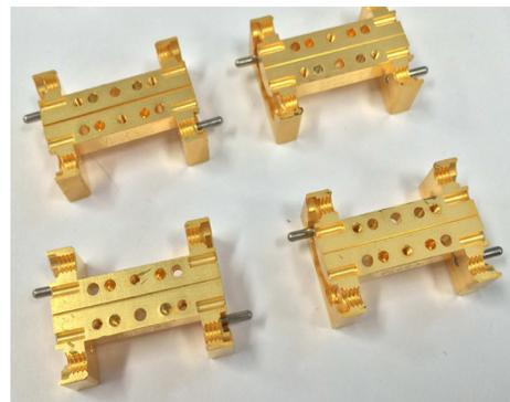
FIG. 1. WR3.4 (left top and bottom) and WR1.5 (right top and bottom) 25 mm long waveguides from VDI made of Al with thin gold plating.
