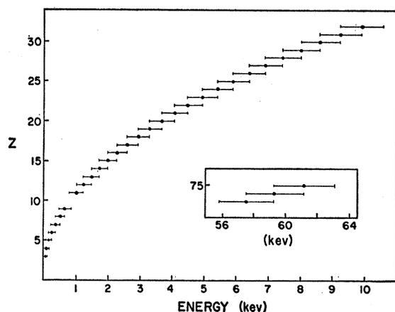
FIG. 1.  $K\alpha$  energies and calculated PHD half-widths as a function of atomic number, based on 15 percent half-width for  $^{20}\text{Cu}$ . Insert shows the half-widths for the  $K\alpha$  of  $^{75}\text{Ta}$ ,  $^{60}\text{W}$ , and  $^{64}\text{Re}$ .
